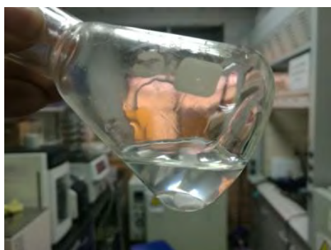
Fig. 1 Solubility test of FR-1 in DMAc (20 wt%)
