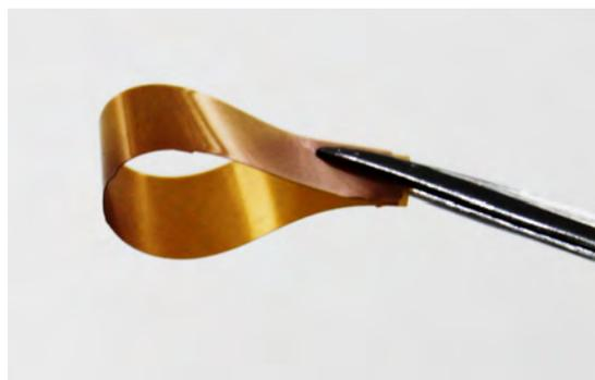
Figure 8. Appearance of the cured polymer alloy film with flexibility (PI/pBXZ=20/80).
