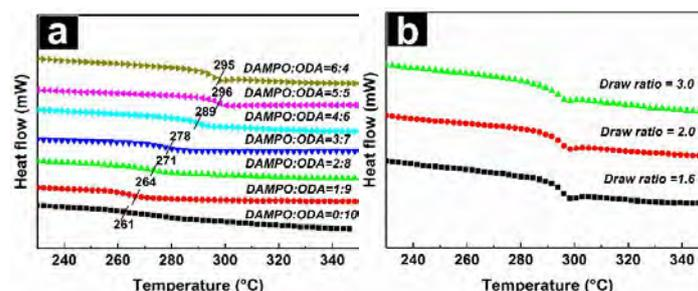
**Figure 1.** DSC spectra of PI fibers with DAMPO ratios (a) and draw ratios (b).
