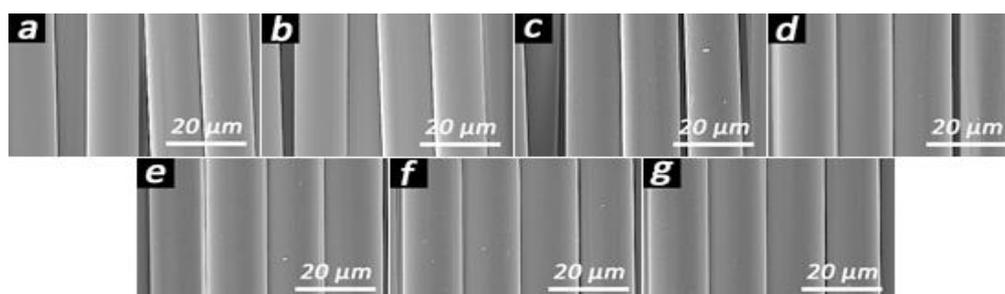
Figure 3. Surface morphologies of fibers (a-g corresponding to PI-0 to PI-6).
