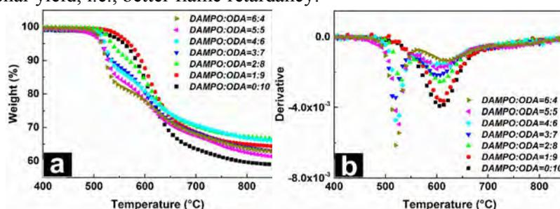
**Figure 2.** TGA and their derivative curves of co-PI fibers.
