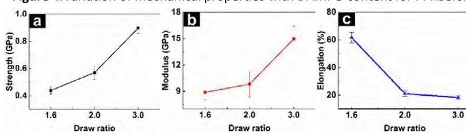
Figure 5. Variation of mechanical properties with draw ratio of co-PI fibers.
