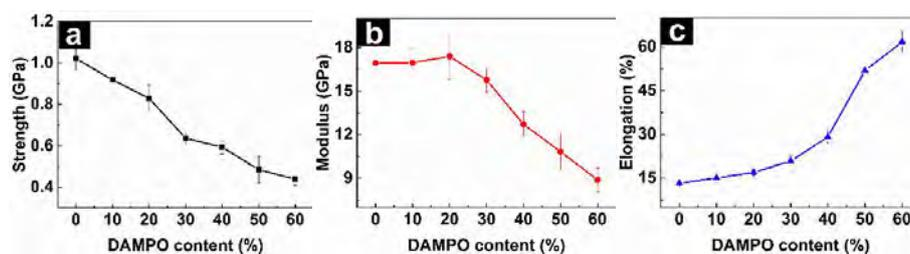
Figure 4. Variation of mechanical properties with DAMPO content for PI fibers.
