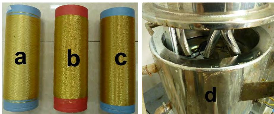
**Figure 4.** Polyamide acid (a), polyimide (b, c) fibers and aggregation apparatus (d).
