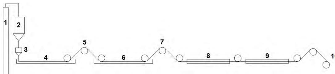
**Scheme 2.** Process of spinning polyamide fibers. 1. Air compressor; 2. Polyamide acids solution; 3. Spinning spinneret; 4. Coagulation bath; 5 and 7. Rollers; 6. Washing bath; 8. Drying-tube; 9. Heating-tube with 340 °C; 10. Winder.
