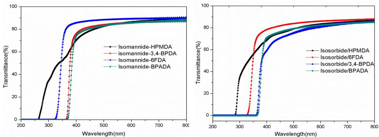
Figure 1. UV-Vis spectra of biobased polyimides
