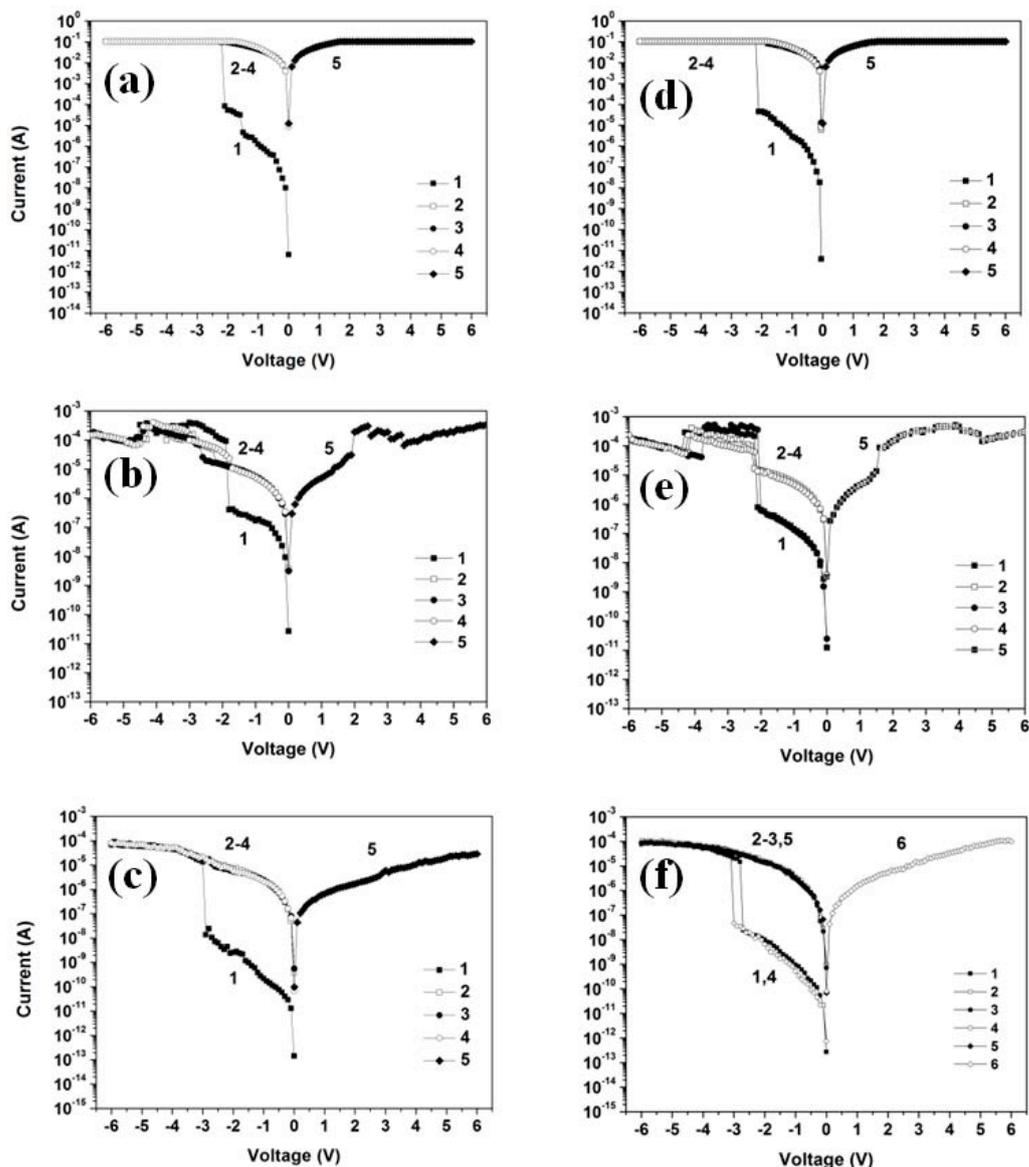
**Figure 1.** Current-voltage (I-V) characteristic of (a) ITO/OI(APAP-6FDA) (38 nm)/Al device, (b) ITO/OI(APAP-6FDA) (48 nm)/Al device, (c) ITO/OI(APAP-6FDA) (85 nm)/Al device, (d) ITO/OI(APAN-6FDA) (38 nm)/Al device, (e) ITO/OI(APAN-6FDA) (48 nm)/Al device, and (f) ITO/OI(APAN-6FDA) (85 nm)/Al device.
