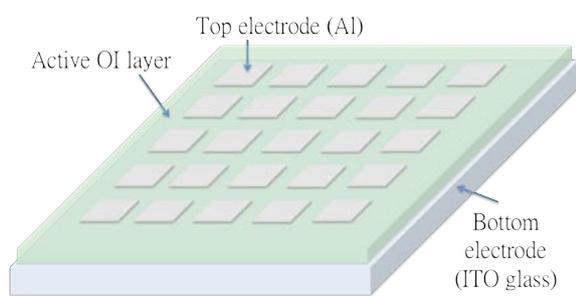
**Figure 2.** Schematic memory device architecture.
