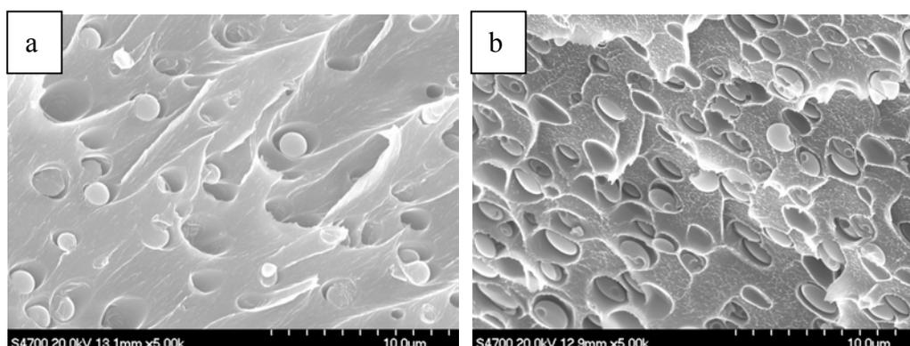
Figure 5. SEM micrograph for PI/SPPSQ(90/10) thermally treated at 100°C (a) and 200°C (b)
