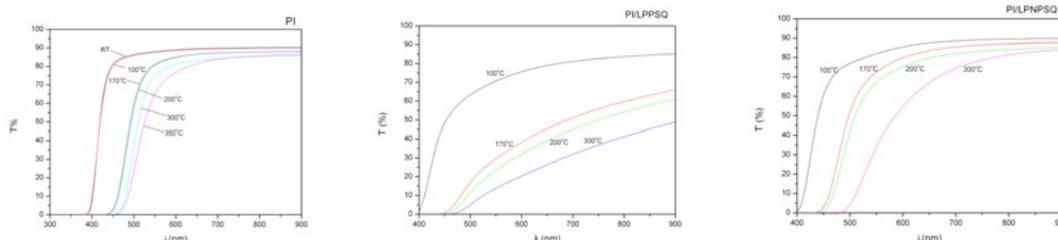
Figure 4. UV-vis spectra of pure PI, PI/SPPSQ(90/10) and PI/SPNPSQ(90/10) hybrid films at different temperature
