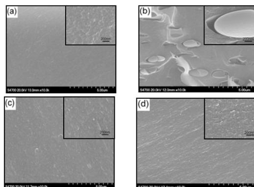
Figure 3. SEM micrographs of (a) pure PI, (b) PI/LPPSQ, (c) PI/LPNPSQ, and (d) PI/LPAPSQ hybrid films
