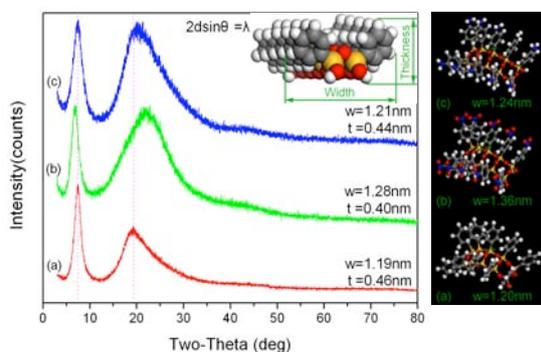
Figure 2. XRD patterns and molecular simulation images of (a) LPPSQ, (b) LPNPSQ and (c) LPAPSQ
