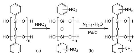
Figure 1. Reaction scheme and their structures of LPPSQ to LPNPSQ and LPAPSQ
