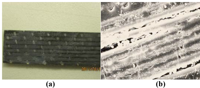
Figure 4. (a) Image of the composite material after radiation (b) SEM images of the composite materials after radiation
