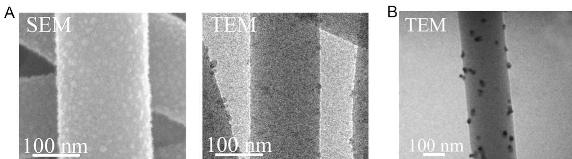
**Figure 2.** (A) SEM and TEM images for the ultrafine PI-Ag fibers prepared via the direct ion exchange process. The PAA fibers were ion-exchanged in a 0.01 M aqueous  $[Ag(NH_3)_2]^+$  solution for 20 s followed by thermal treatment to 300 °C for 2h in N<sub>2</sub>. (B) TEM images for the PI-Ag nanohybrid fibers (2 wt% Ag) prepared via the in-situ single stage self-metallization process using AgTFA as the silver precursor.
