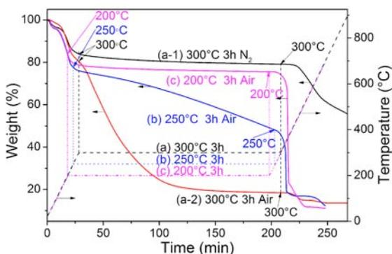
**Figure 3.** The isothermal TGA curves measured at different temperatures in nitrogen and air atmospheres for the PAA ultra fine fibers ion exchanged in a 0.01 M aqueous  $[Ag(NH_3)_2]^+$  solution for 20 s.
