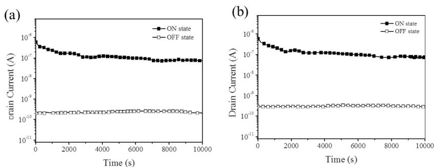
**Figure 5.** Retention time testing of the OFET memory devices based on BPE-PTCDI thin film with (a) PI(APSP-6FDA) and (b) PI(APST-6FDA) as electrets.
