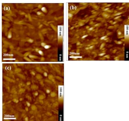
**Figure 3.** AFM topographic images of pentacene on different polymer surface: (a) PI(APSP-6FDA), (b) PI(APST-6FDA) and (c) PI(ODA-6FDA) on 1  $\mu\text{m}$  x 1  $\mu\text{m}$  area.
