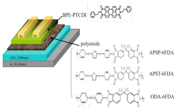
**Figure 2.** Schematic structure of the BPE-PTCDI thin film based OFET memory device.
