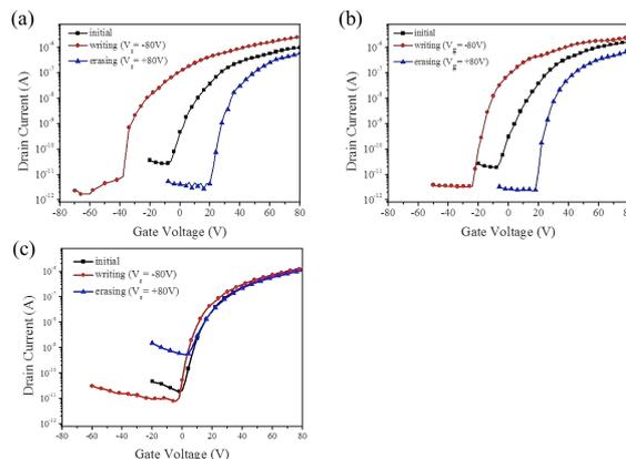
**Figure 4.** Shifts in transfer curves for BPE-PTCDI OFET memory device with (a) PI(APSP-6FDA), (b) PI(APST-6FDA) and (c) PI(ODA-6FDA) as polymer electrets.
