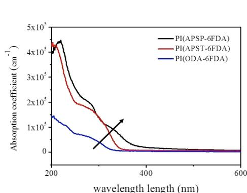
**Figure 1.** UV-vis absorption spectra of PIs
