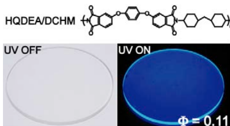
Figure 2. Photos of a highly fluorescent polyimide films on silica substrates without/with UV irradiation.
