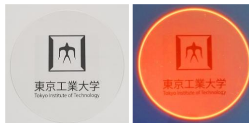
Fig. 6 Photographs of a large size film of CoPI-0.03 doped with 2eq \text{H}_2\text{SO}_4 formed on the soda glass substrate. Left: under sunlight. Right: under 375 nm UV light.
