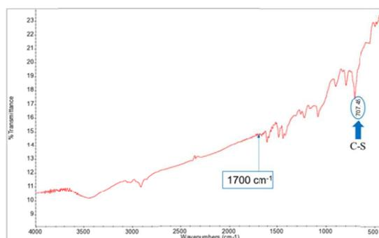
Figure 6 FT-IR spectrum of poly (m-xylylene sulfide) was synthesized at TMDS 24 mmol
