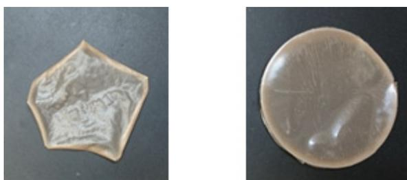
**Fig. 1** Photographs of (left) the composite membranes with PL1-based nanoparticles and (right) Stöber-based nanoparticles
