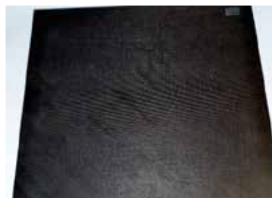
Figure 1. Carbon fiber/TriA-X composite material prepared by in situ PMR method (200×200mm, V_f=55\% )
