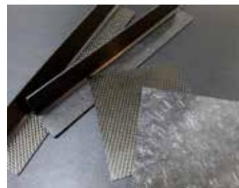
Fig.1 PEI/CF composite derived from paper making technologies.
