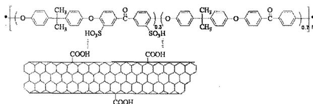
**Scheme 1.** Synthesis of Sulfonated Poly(Aryl ether ketone) copolymers and *a*-MWNTs/SPAEK composite membranes.
