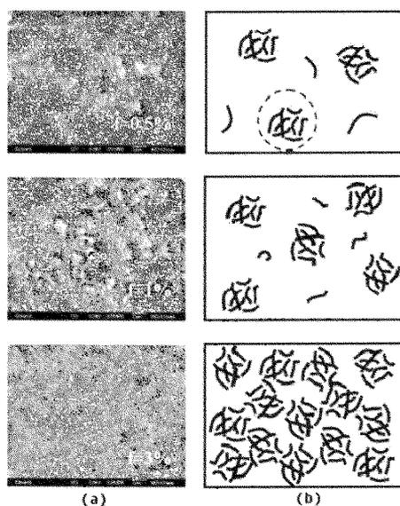
**Figure 1.** (a) Scanning electron microscopy image illustrating the morphology of a section of the a-MWNTs/SPAEEK nanocomposite with the a-MWNTs volume fraction of 0.005, 0.01 and 0.03. (b) Schematic pictures of a-MWNTs distribution in polymer composites at different concentrations of a-MWNTs.
