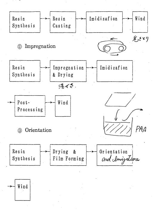
Some properties of PI film relate to the producing process, such as tensile strength, dielectric strength, dissipation factor. Among them, tensile strength is the most influenced. (Tab. 1)
