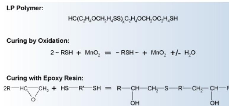
**Figure 1 :** Conventional polysulfide structure and hardener
