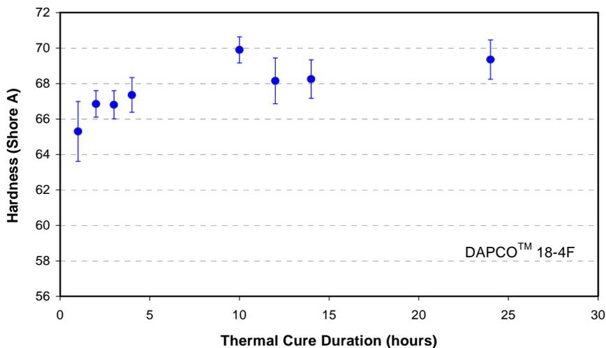
**Figure 3.** Hardness versus cure time results for DAPCO 18-4F sealant cured at 65°C.
