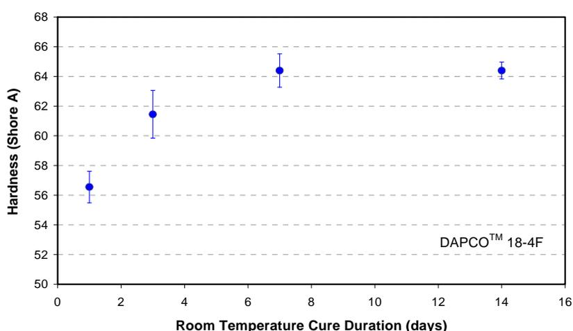
**Figure 2.** Hardness against cure time results for DAPCO 18-4F sealant cured at room temperature.
