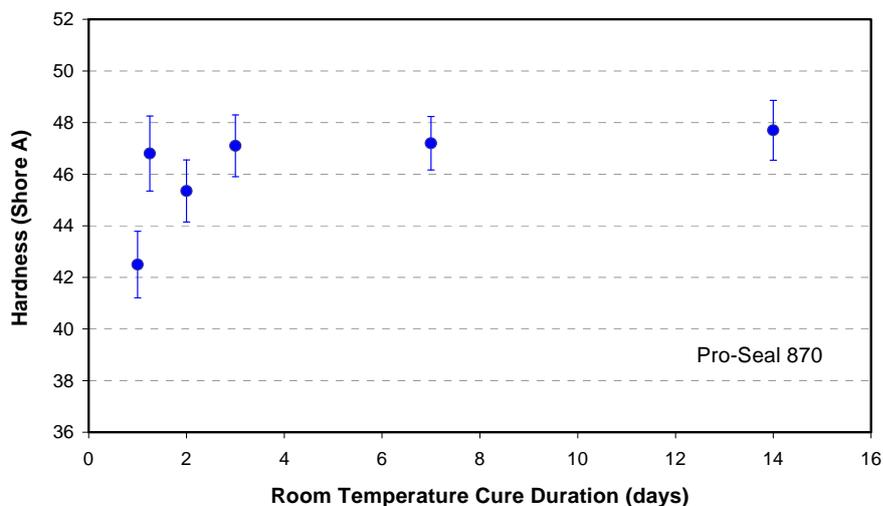
Figure 5. Hardness versus cure time results for Pro-Seal 870 sealant cured at room temperature.
