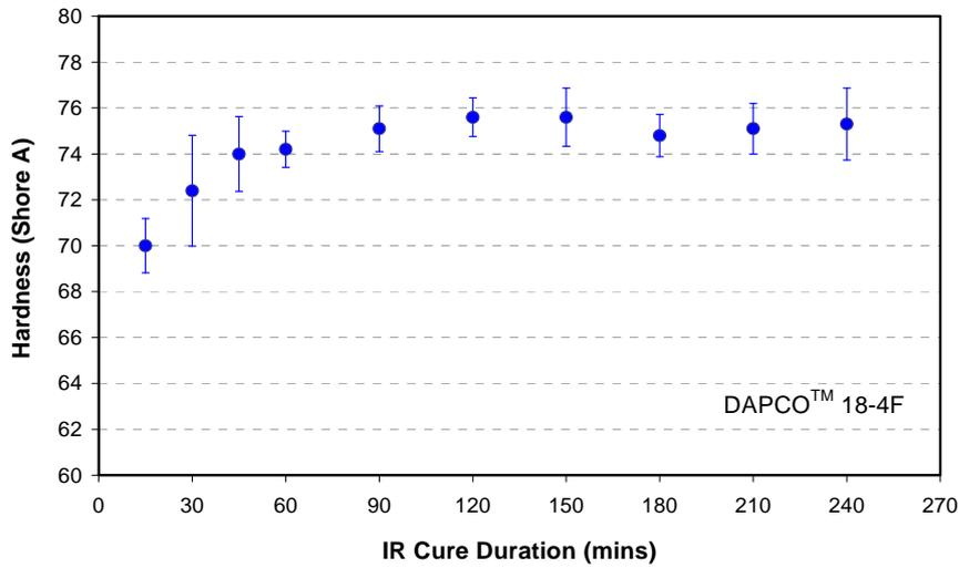
Figure 4. Hardness versus cure time results for DAPCO 18-4F sealant cured via IR.
