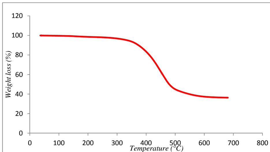
**Figure 5 :** Thermogravimetric Analysis of Empty Silica Gels Microcapsules
