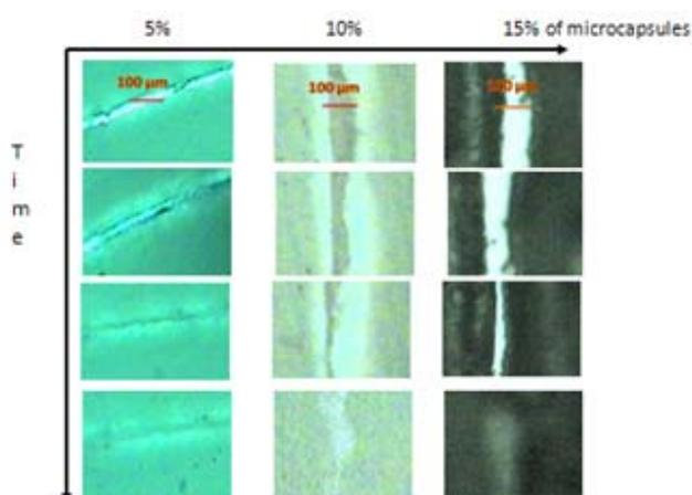
Figures 9 and 10 show the reconstitution of the Polyimide film for different concentration of silica-gel microcapsules versus time of exposure to UV radiation, 0 min, 5 min, 10 min and 15 min respectively for intensity of 100 mW/cm<sup>2</sup>.
