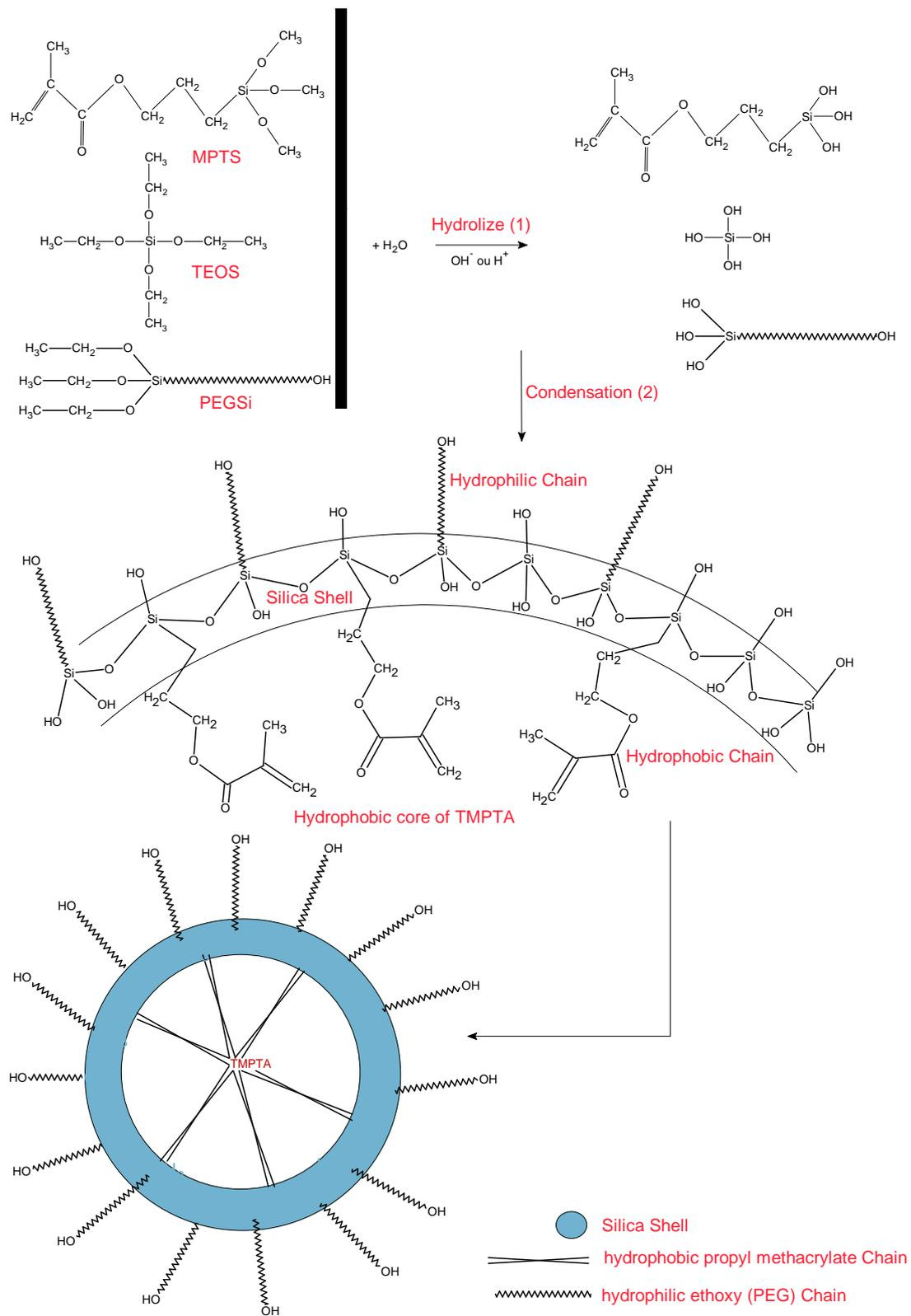
**Figure 3.** Schematic Road for Synthesis of Silica Gel Microcapsules Loaded in TMPTA
