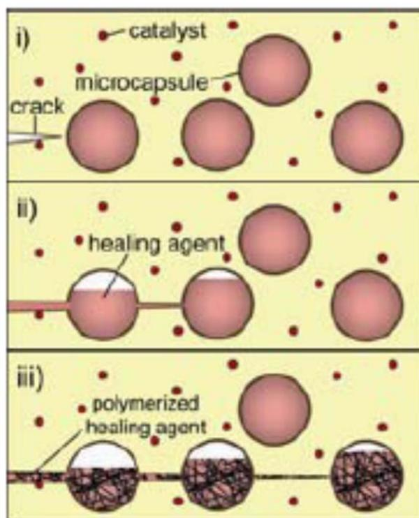
**Figure 1.** Concept of reservoirs developed by White S. R et al
