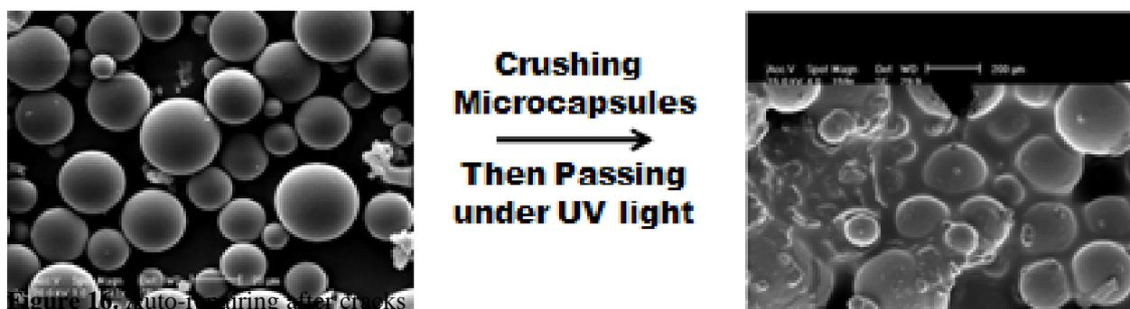
Figure 8. Effect of UV after cracking micro-gel capsules on Polyimide film
