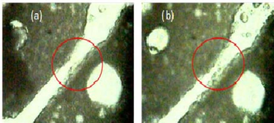
**Figure 10.** Cracks at time zero (a) – Cracks at exposure time 5 min
