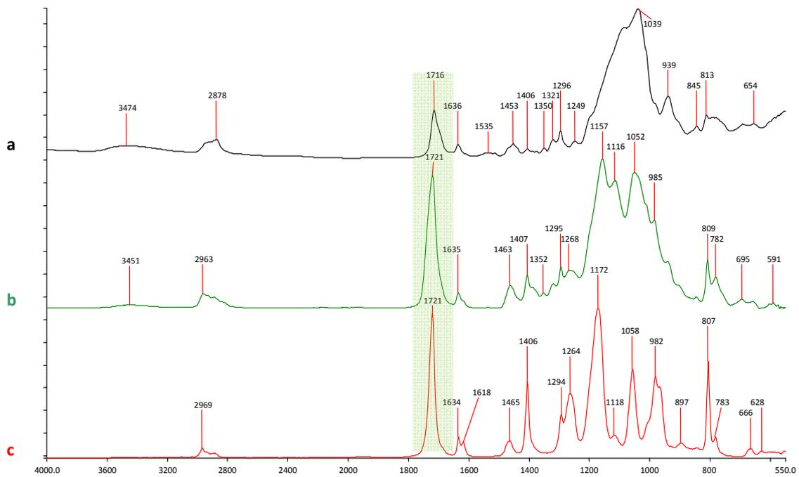
**Figure 4.** Infrared spectrum of (a) Empty silica gels microcapsules (b) silica gels microcapsules loaded in TMPTA monomer and (c) TMPTA
