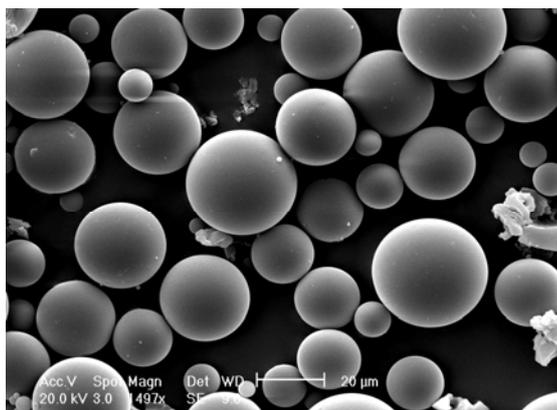
**Figure 3.** ESEM image of Silica gels microcapsules loading in TMPTA monomer and Darocur ®1173 photoinitiator
