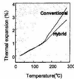
Fig. 9.2 Temperature dependency of thermal expansion
