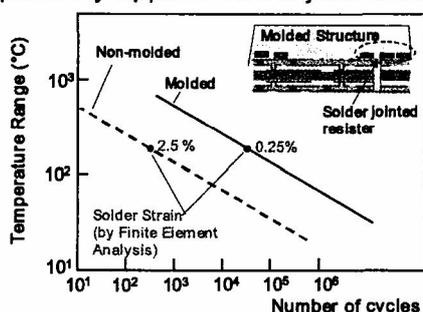
Fig. 6 Reliability of Solder Joints of Resistor
