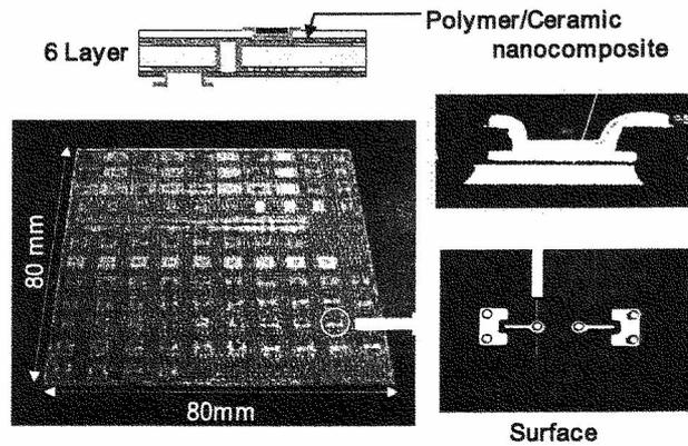
Fig. 15 6-layer Wiring substrate with embedded capacitor
