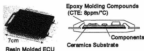
Fig. 7 Resin Molded ECU
