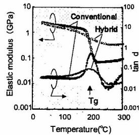
Fig. 9.1 Temperature dependency of elastic modulus
