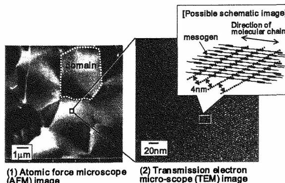
Fig. 12 Nanoscopic and mesoscopic images of high-order structures
