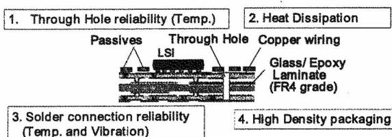
Fig. 5 Cross sectional view of Electronic Control Unit
