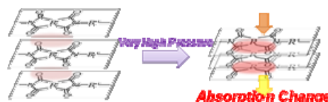
Figure 1. Schematic illustration of change in the aggregation structure under very high pressure.
