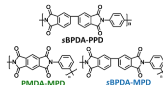
Fig. 1 Molecular structures of PIs.
